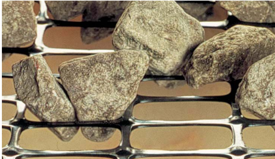
Figure 7 – Tensar Biaxial Geogrid – not just a geotextile
