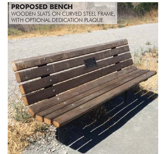
PROPOSED BENCH WOODEN SLATS ON CURVED STEEL FRAME, WITH OPTIONAL DEDICATION PLAQUE
