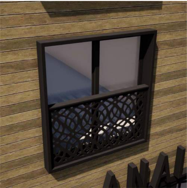
7 ALUMINUM GLAZING SYSTEM EXTENDED FACE-CAP RENDERING WITH PARASOLEIL SCREEN - NO SCALE
