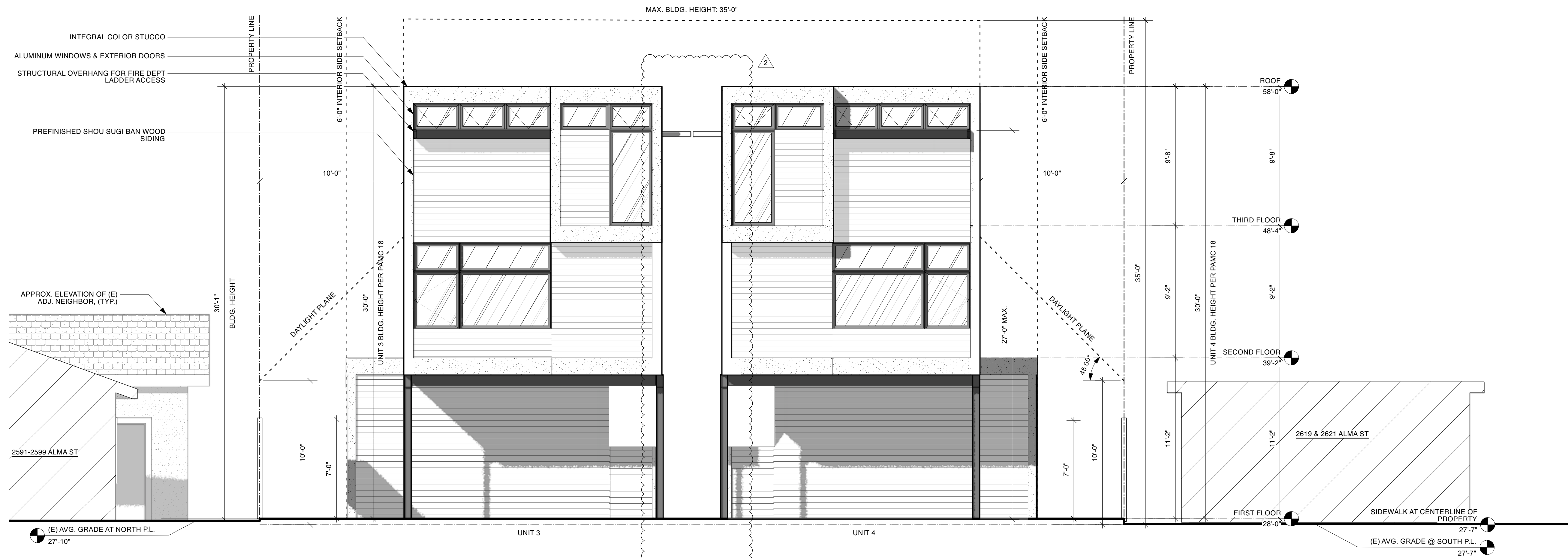
1 A3.03 EXTERIOR ELEVATION - WEST - UNITS 3 & 4 Scale: 1/4" = 1'-0"
