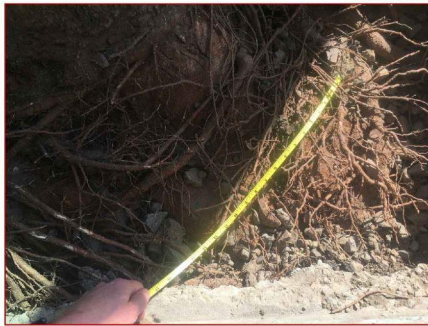
In the above photo, the tape is laid across two roots that combined are 11" across. These roots would require pruning, would be possibly exceed 25% of the total roots on the northwest side of the trunk.
