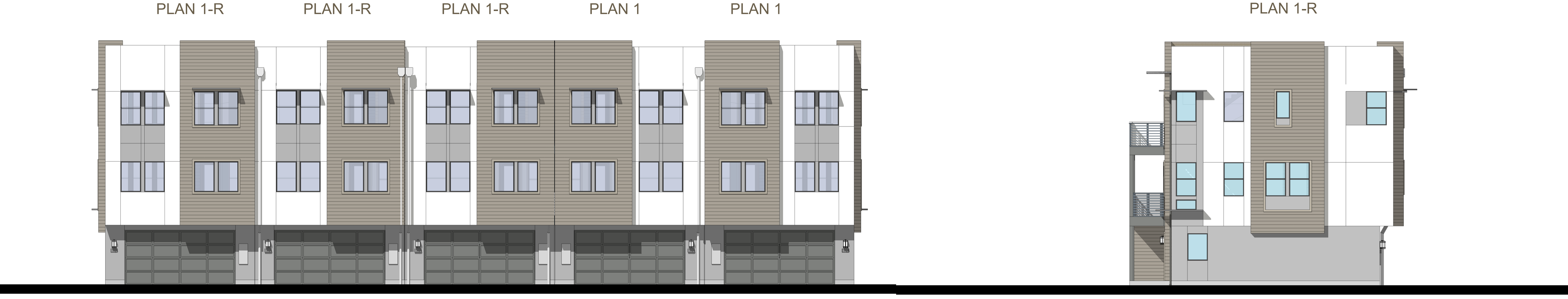
BUILDING 1 - 5 PLEX - REAR ELEVATION SCALE: 1/8"=1'
