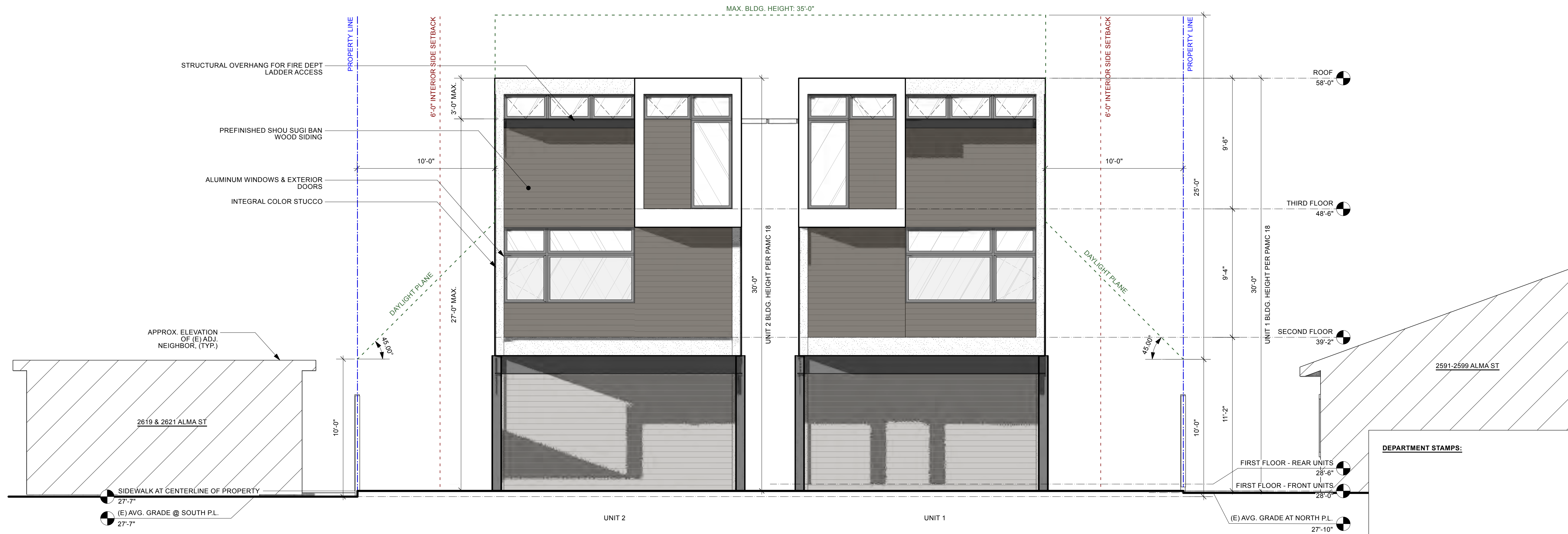
2 A3.03 EXTERIOR ELEVATION - EAST - UNITS 1 & 2 Scale: 1/4" = 1'-0"
