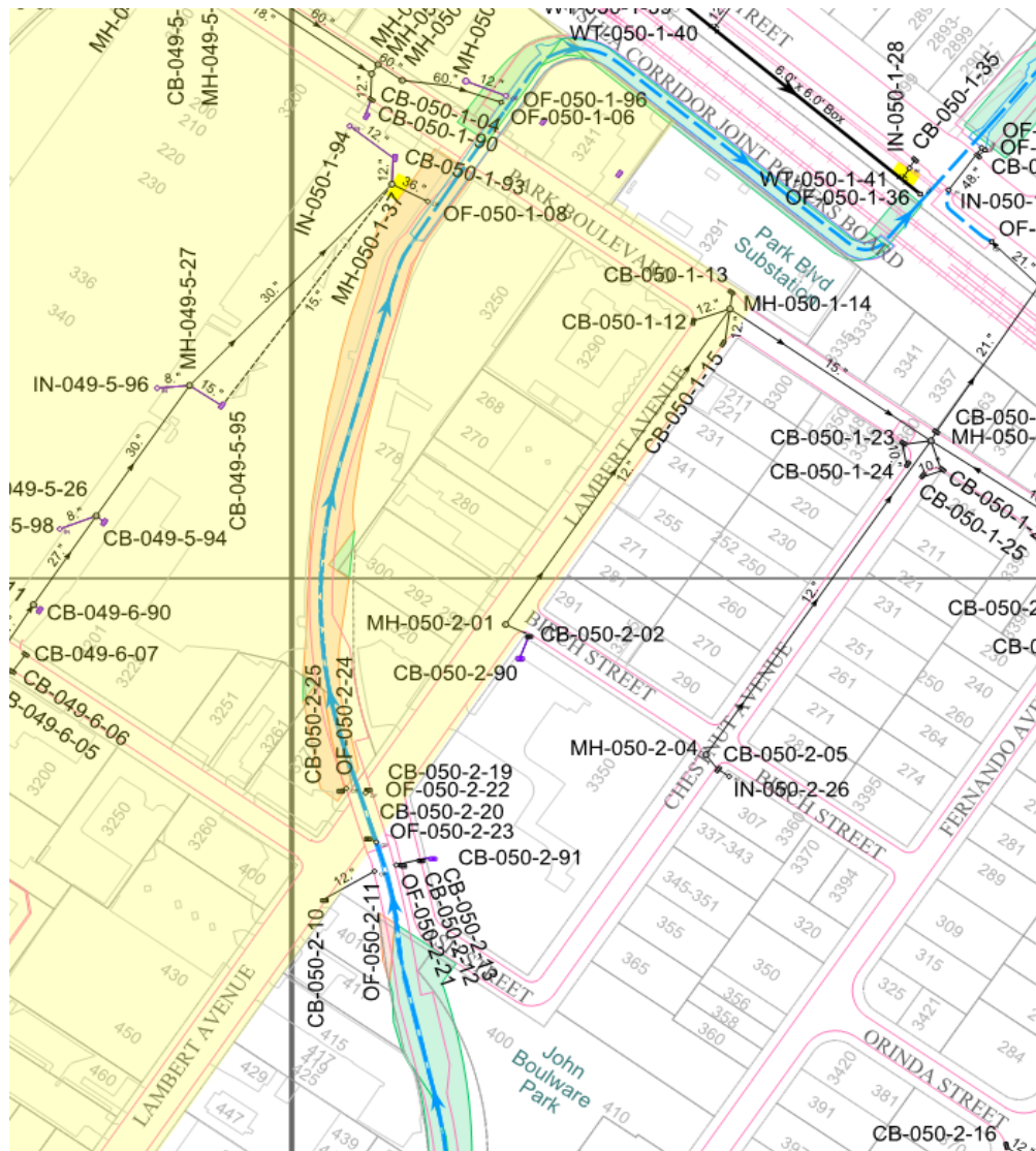
Figure 93 Storm Drain Outfalls to Matadero Creek Channel
