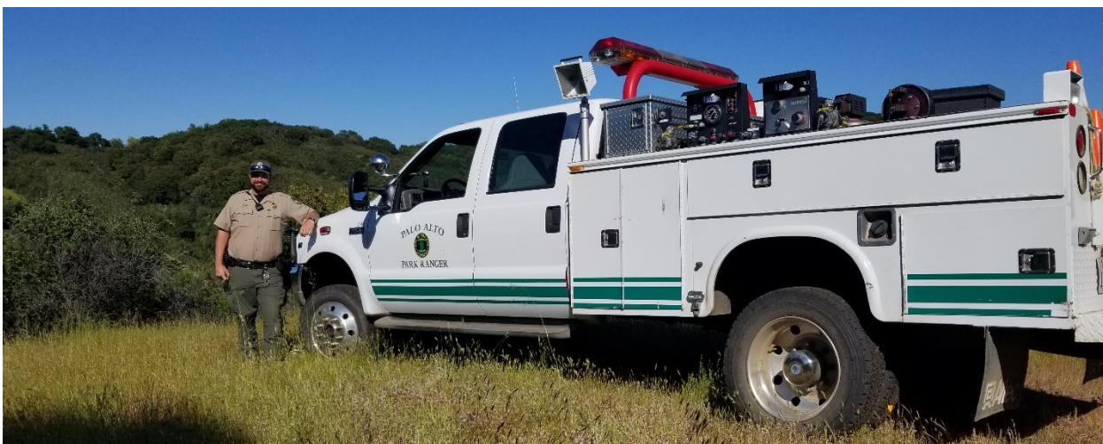
Pickup trucks that meet federal standards as a Type 6 Fire Engine
