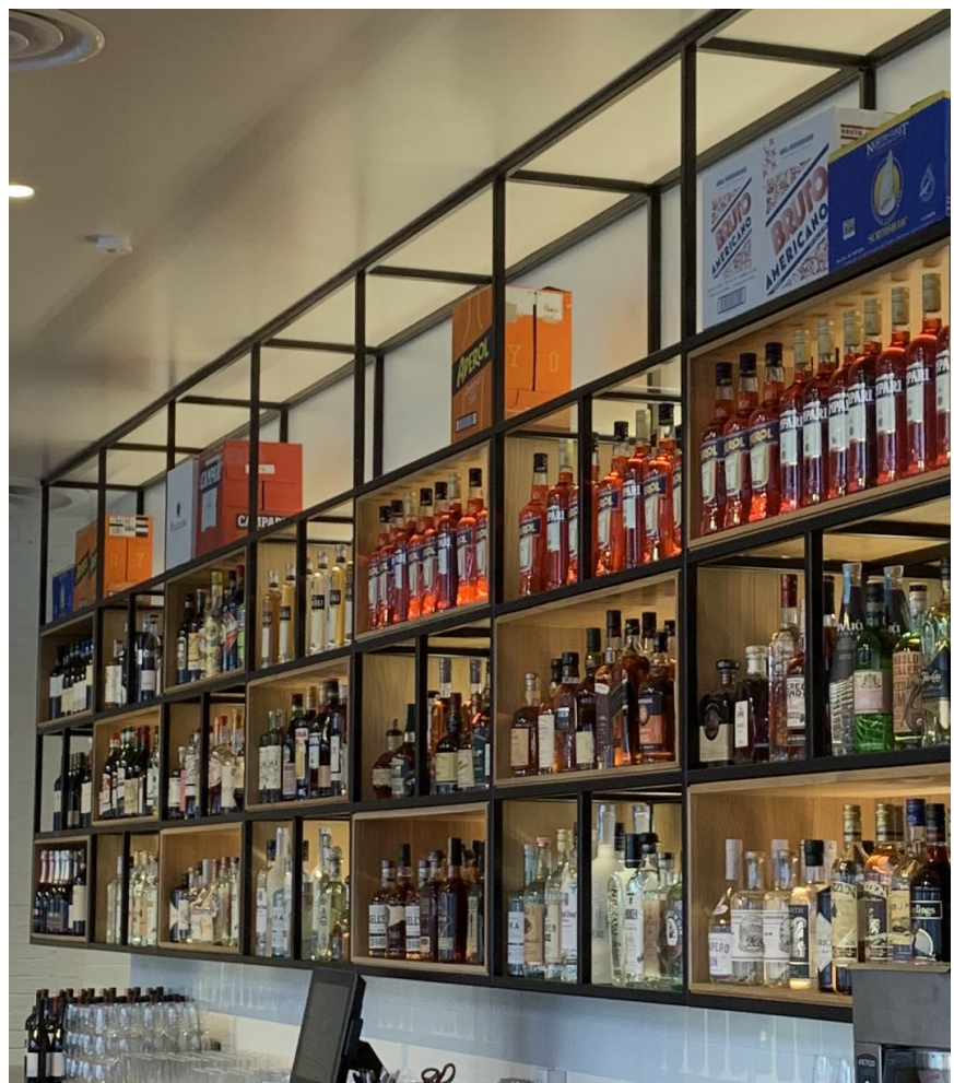
Back bar - 1" black steel tube and glass shelving
