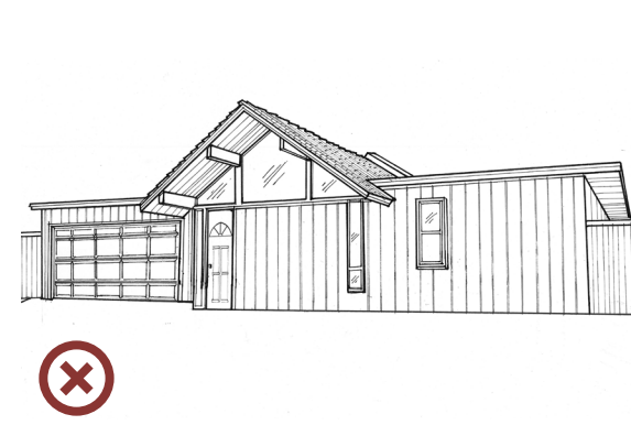
Inappropriate garage door and entry door design for an Eichler home. Panelized garage and entry doors or elaborate glazing are not appropriate for Eichler homes.
