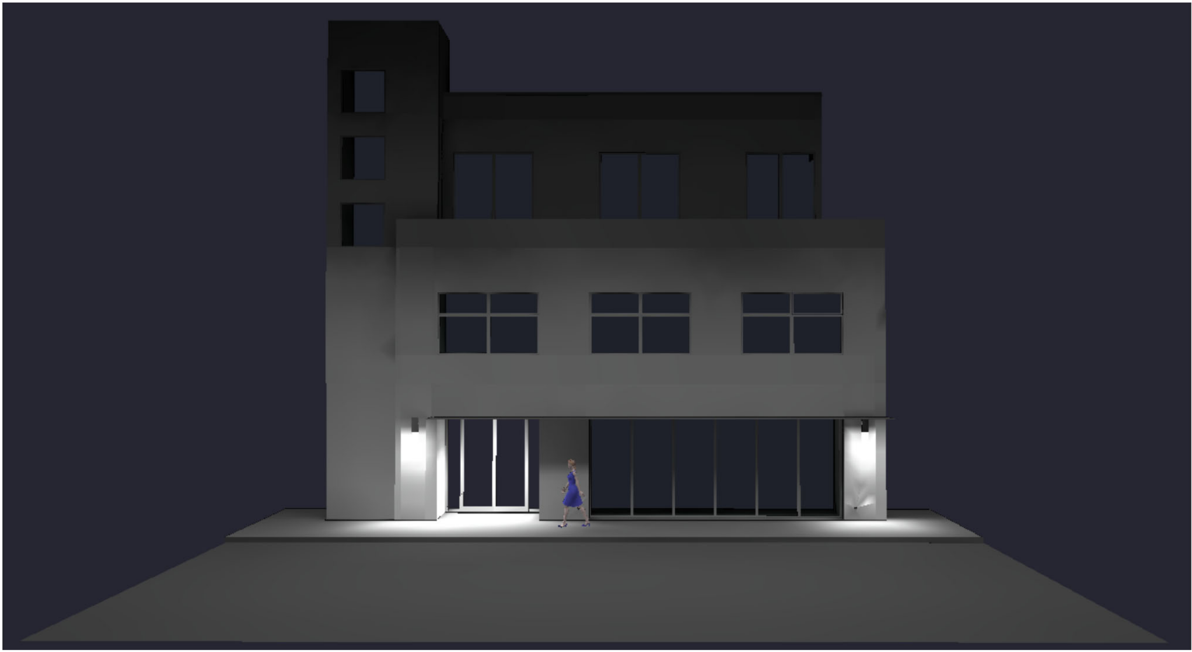
XL1 - LUMENWERX 'AREA-4' RECESSED ROUND DOWNLIGHT 14W 1481 LM BEVEL TRIM SHOWN AT 30% OUTPUT ON EMERGENCY CIRCUIT
