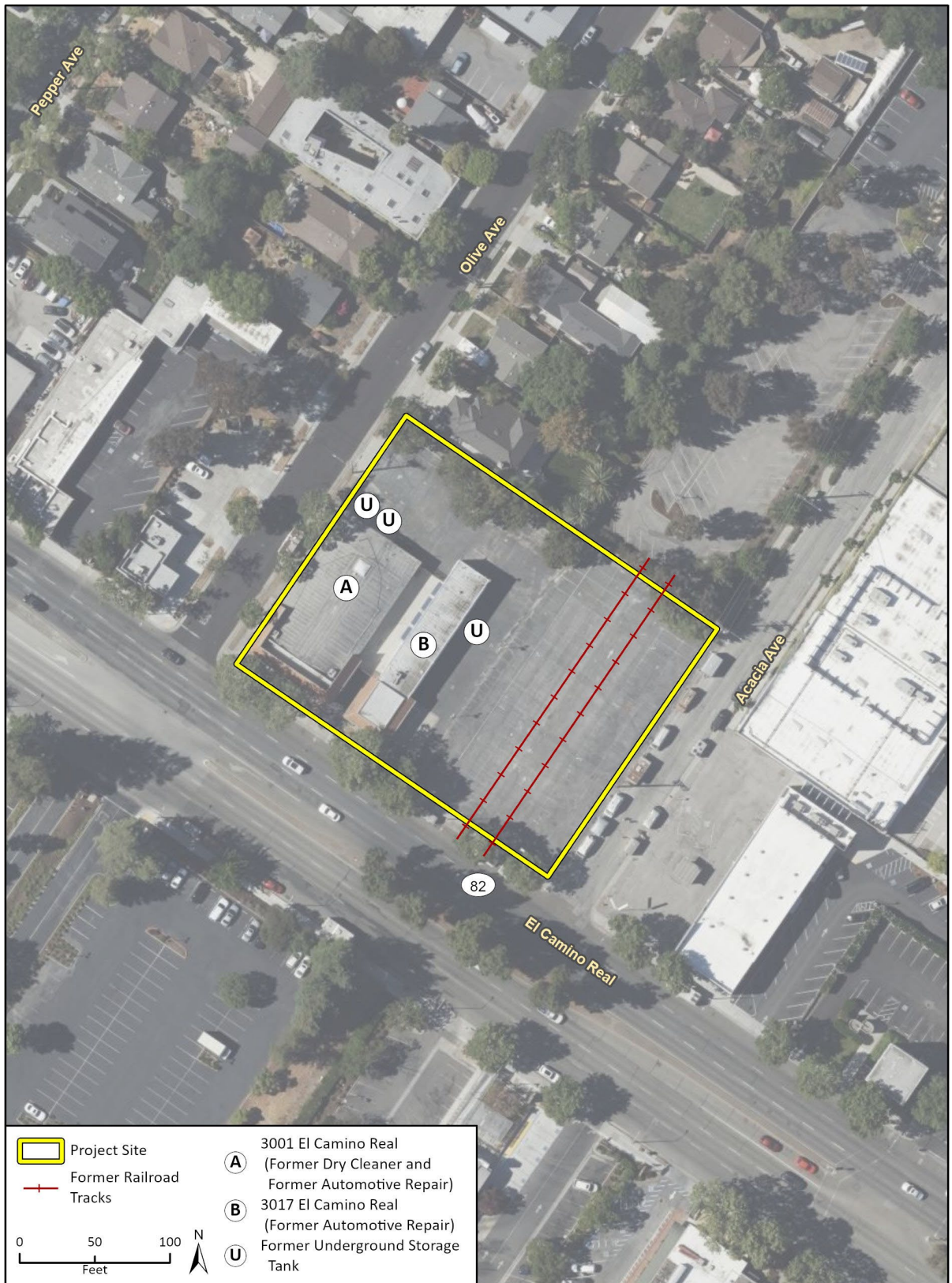
Figure 7 Project Site – Hazardous Materials Concern
