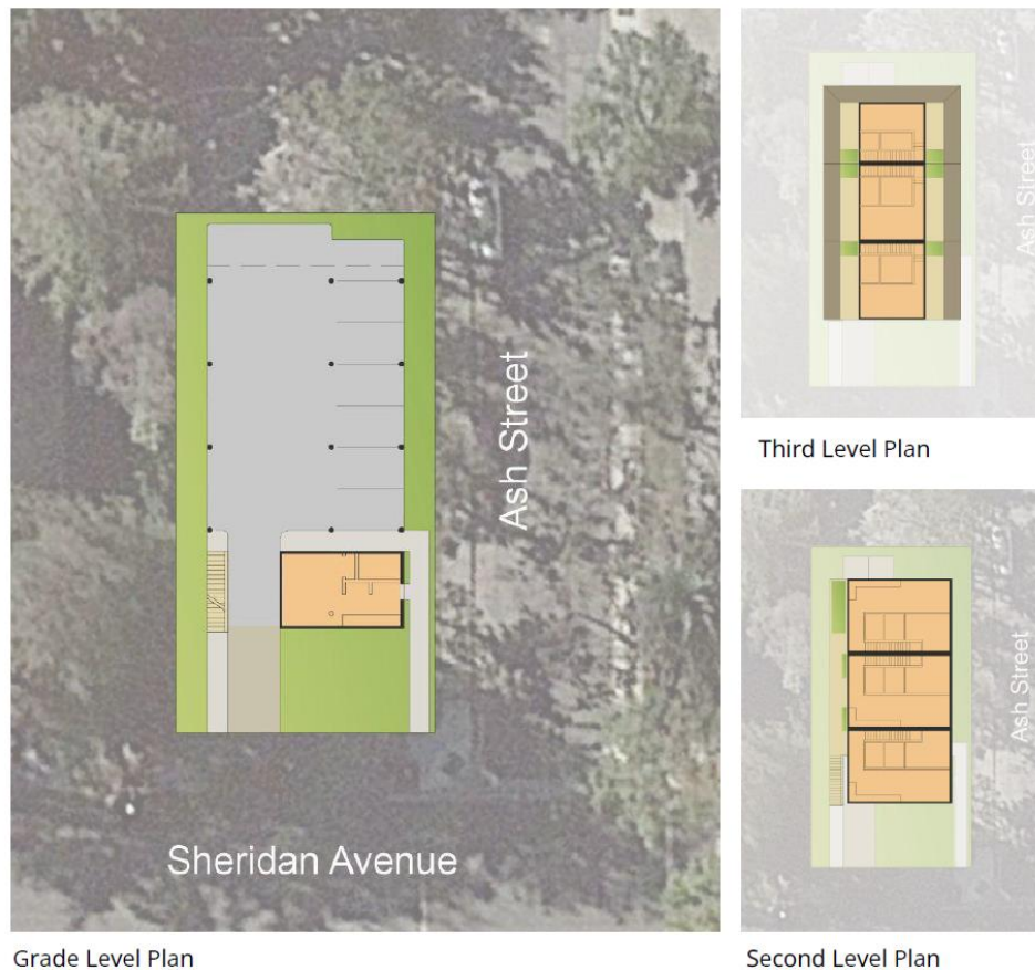
Figure 4-6 RM-40 Zone Model – Parking Compliant with City Code
