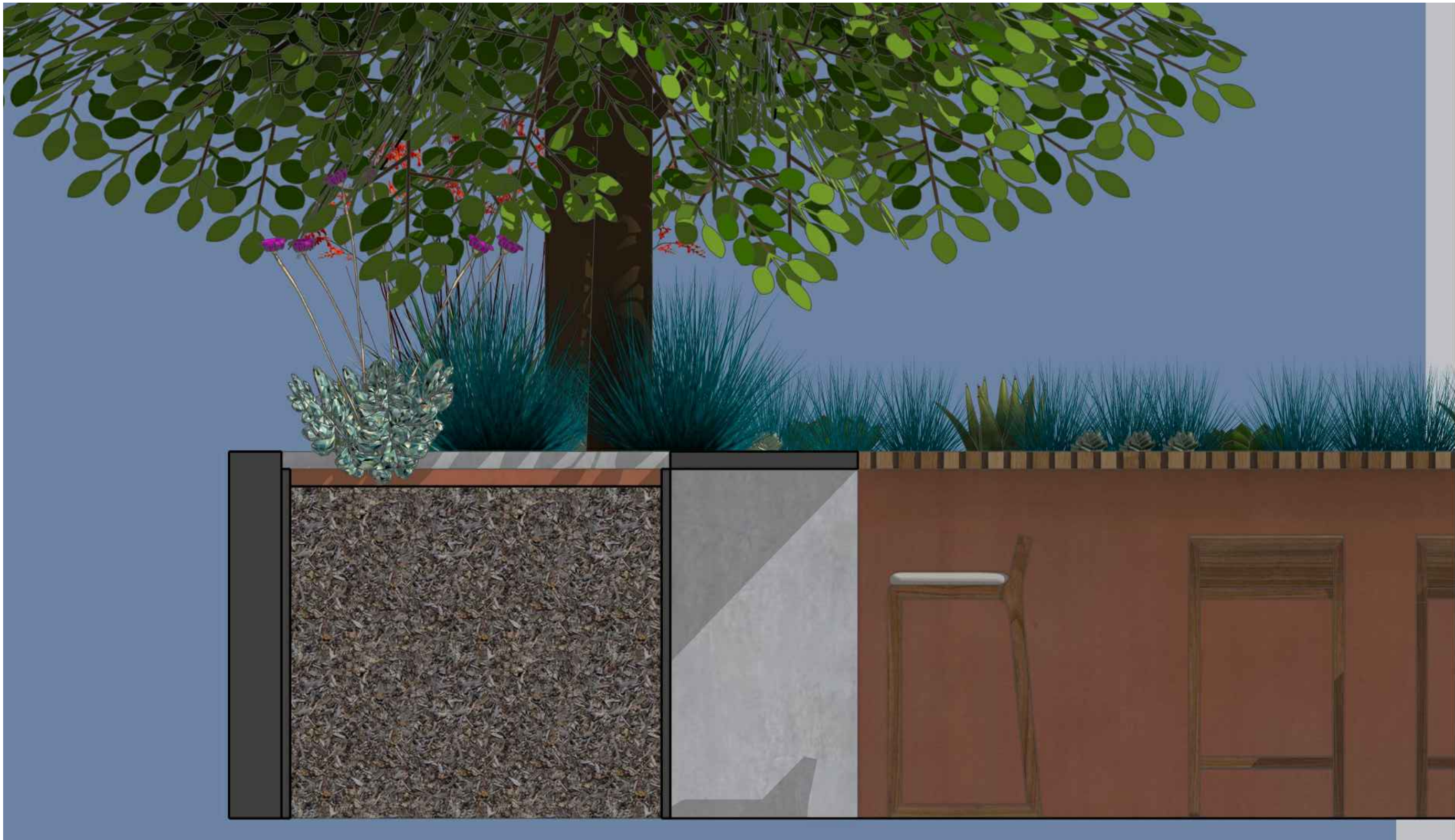
Planter w/ Railing atop Parapet NTS
