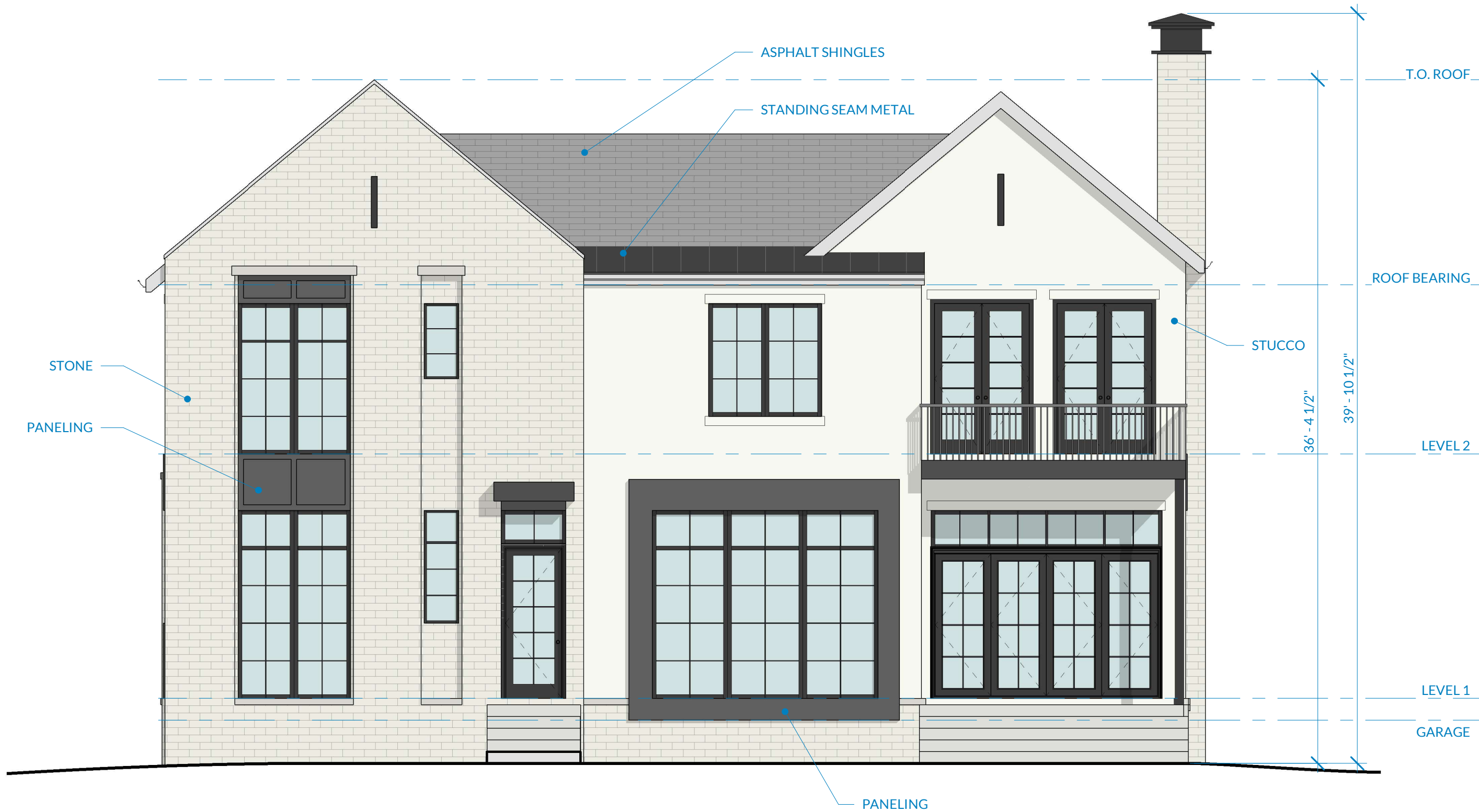
2 LOT 7 - NORTH EXTERIOR ELEVATION (BACK) 3/16" = 1'-0"
