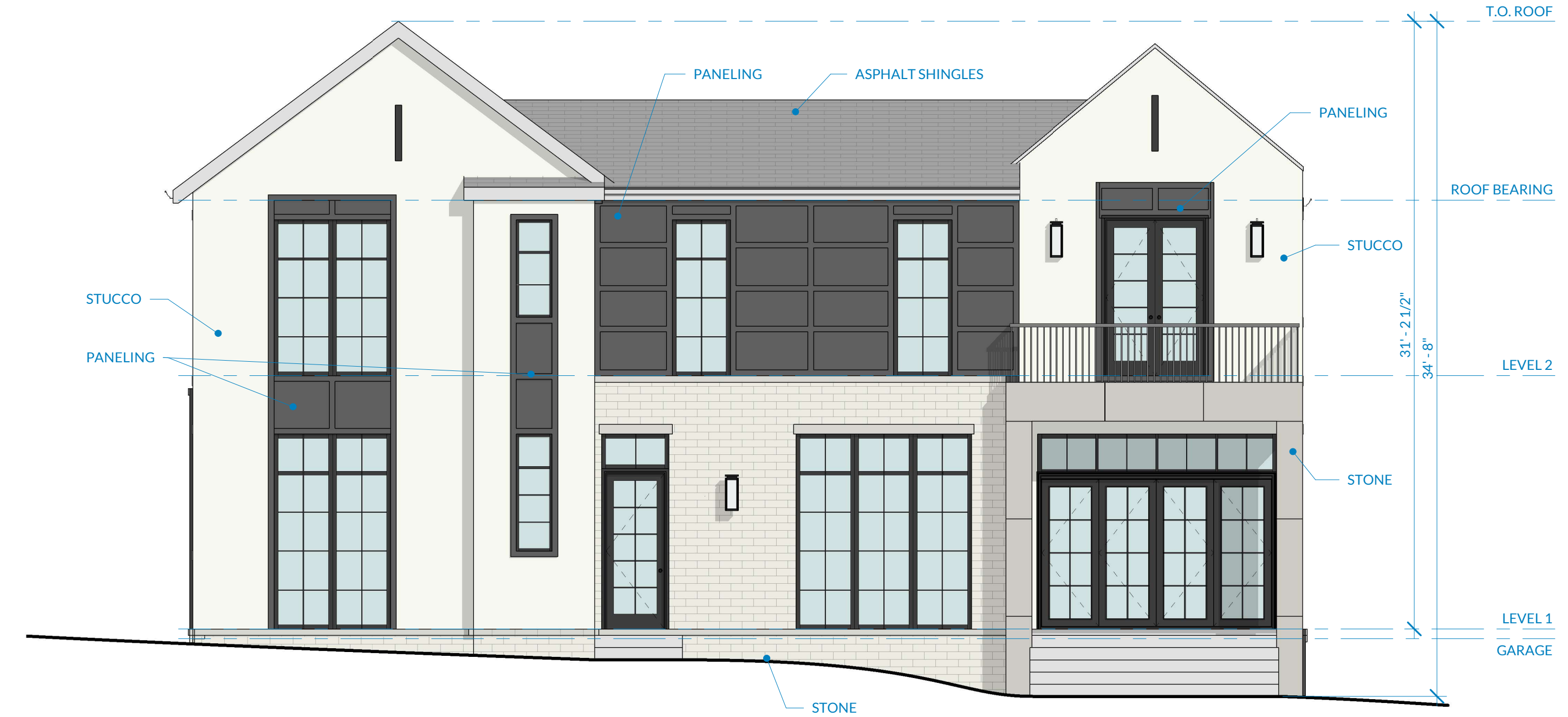
3 LOT 4 - EAST EXTERIOR ELEVATION (BACK) 3/16" = 1'-0"
