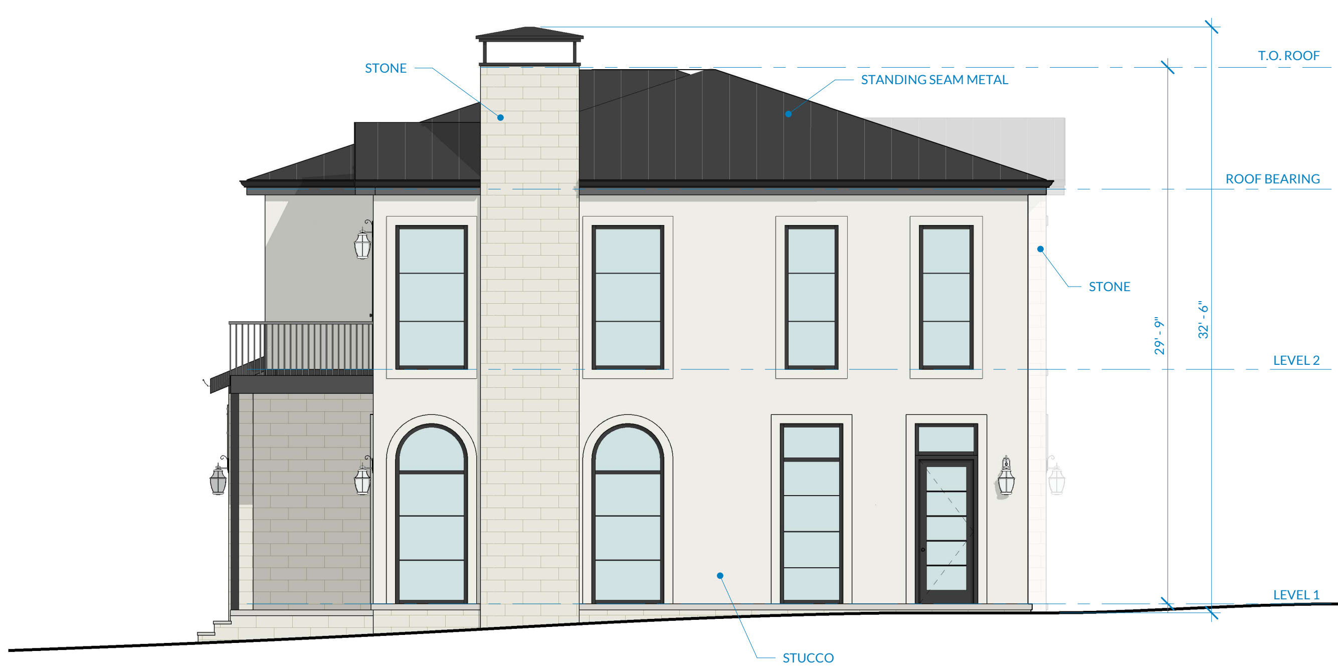
3 LOT 6 - WEST EXTERIOR ELEVATION (SIDE) 3/16" = 1'-0"
