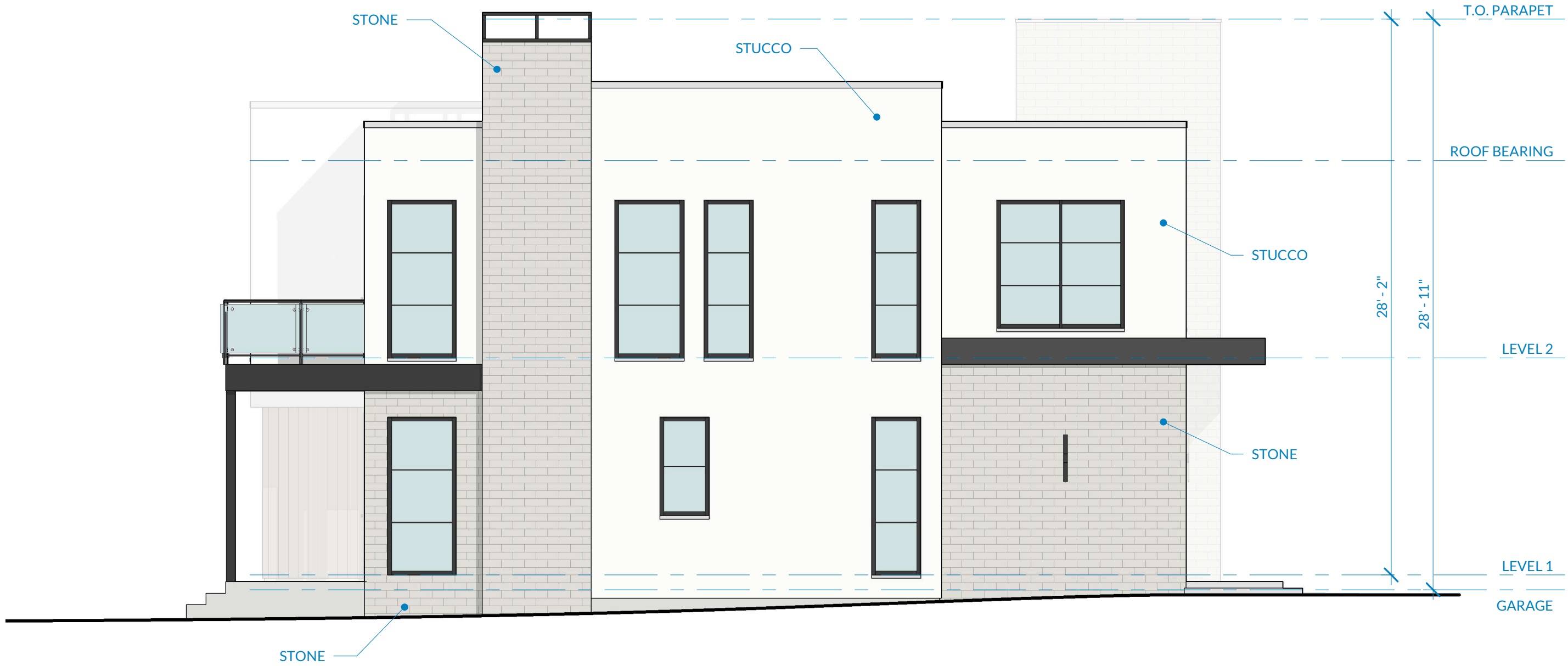
② LOT 5 - NORTH EXTERIOR ELEVATION (SIDE) 3/16" = 1'-0"
