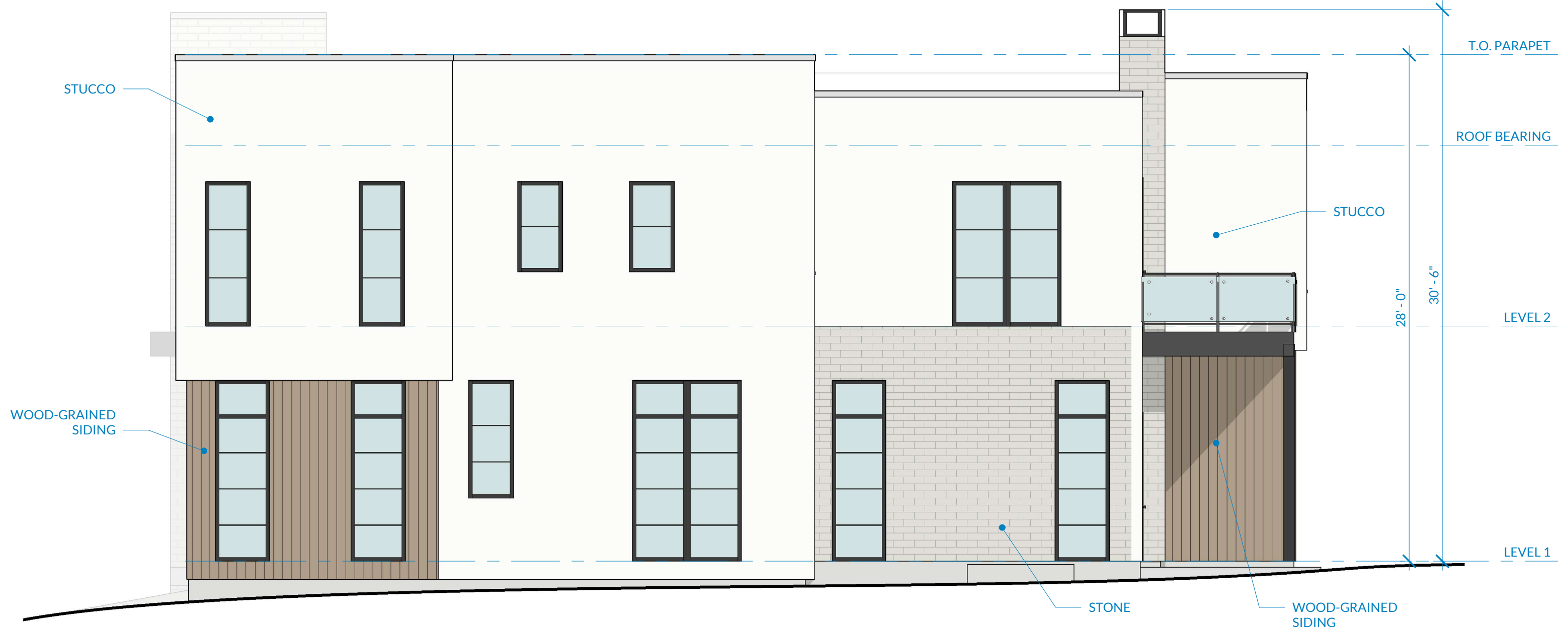
4 LOT 2 - WEST EXTERIOR ELEVATION (SIDE) 3/16" = 1'-0"
