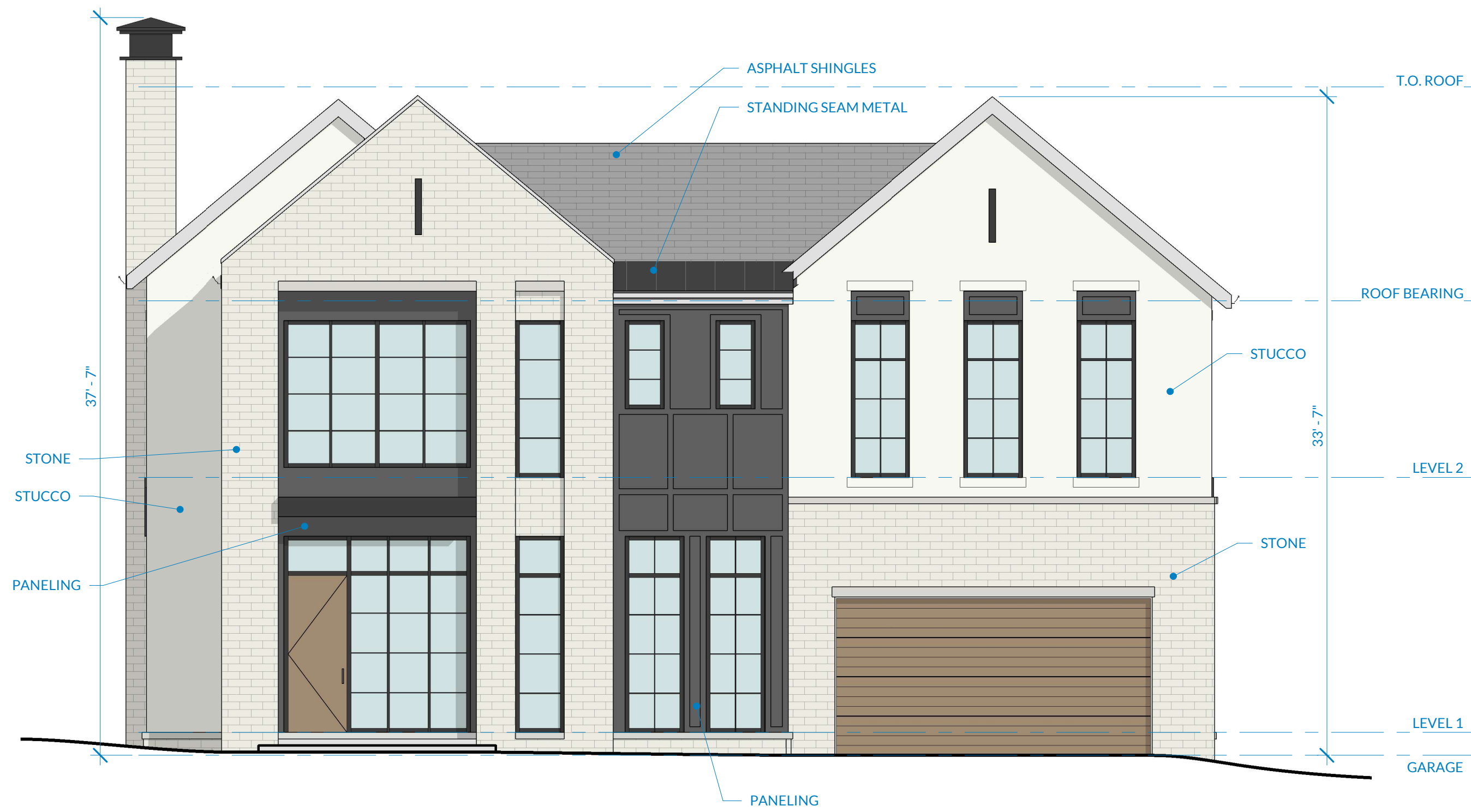
1 LOT 7 - SOUTH EXTERIOR ELEVATIONS (FRONT) 3/16" = 1'-0"
