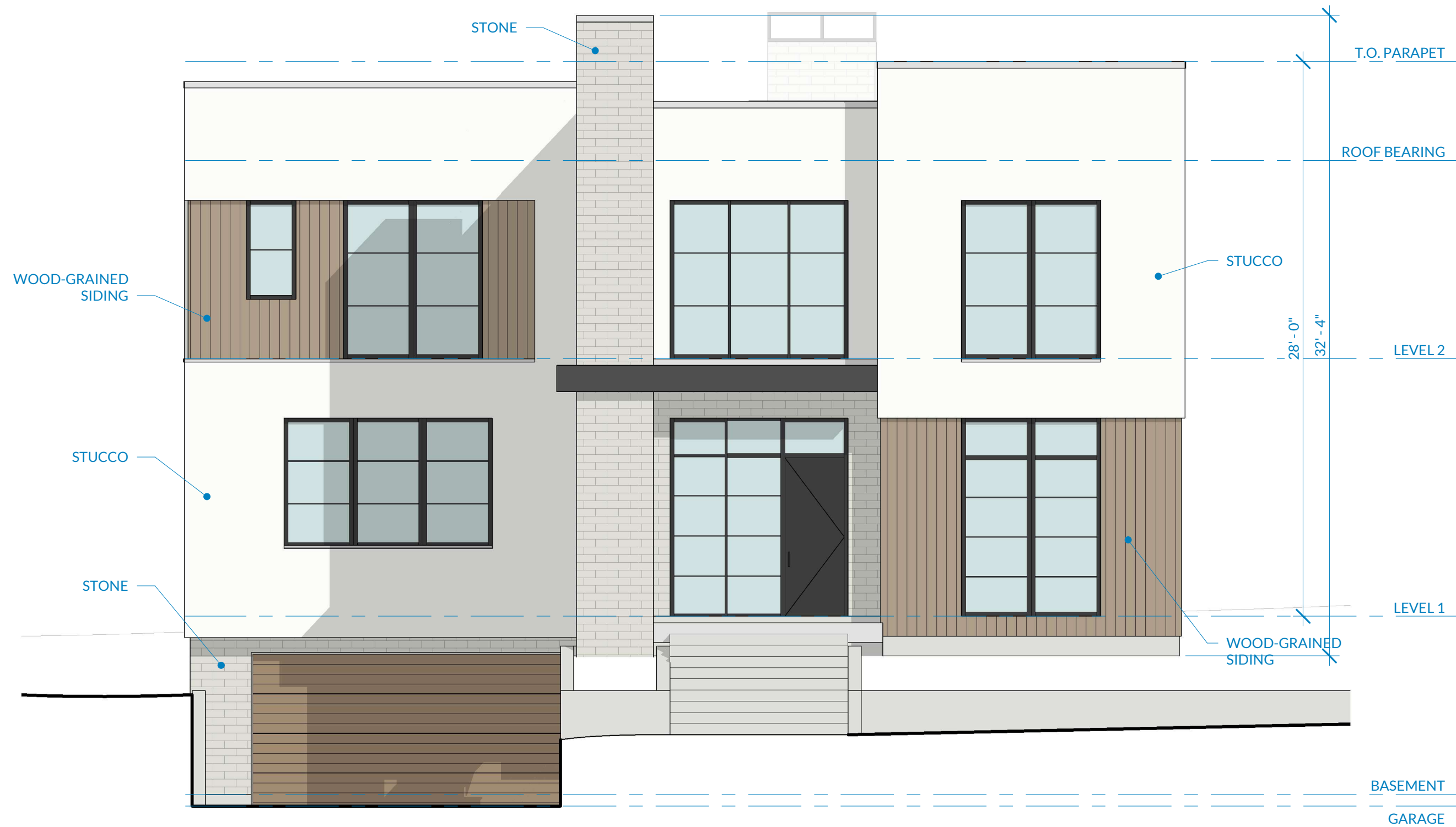
1 LOT 2 - NORTH EXTERIOR ELEVATION (FRONT) 3/16" = 1'-0"
