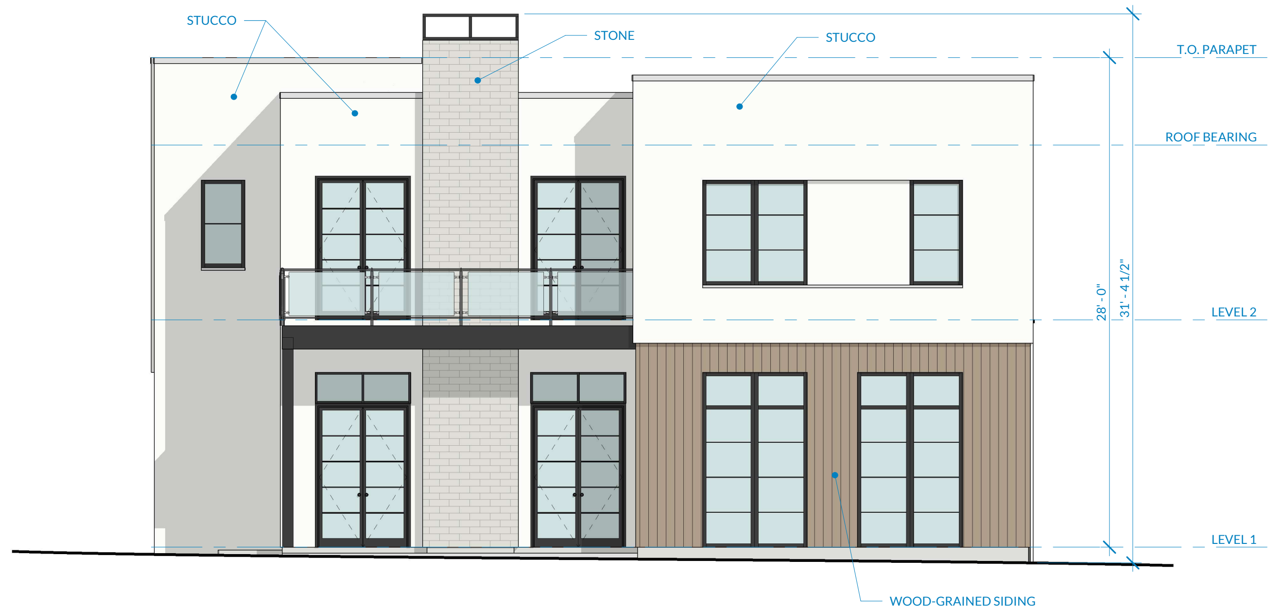
3 LOT 2 - SOUTH EXTERIOR ELEVATION (BACK) 3/16" = 1'-0"
