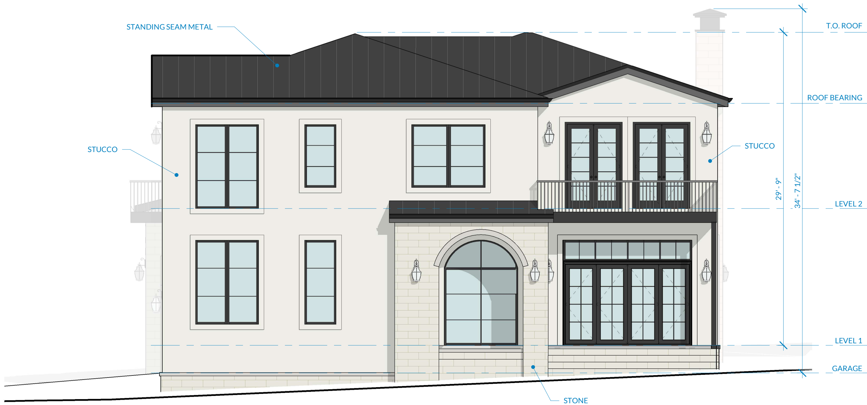
4 LOT 6 - NORTH EXTERIOR ELEVATION (BACK) 3/16" = 1'-0"
