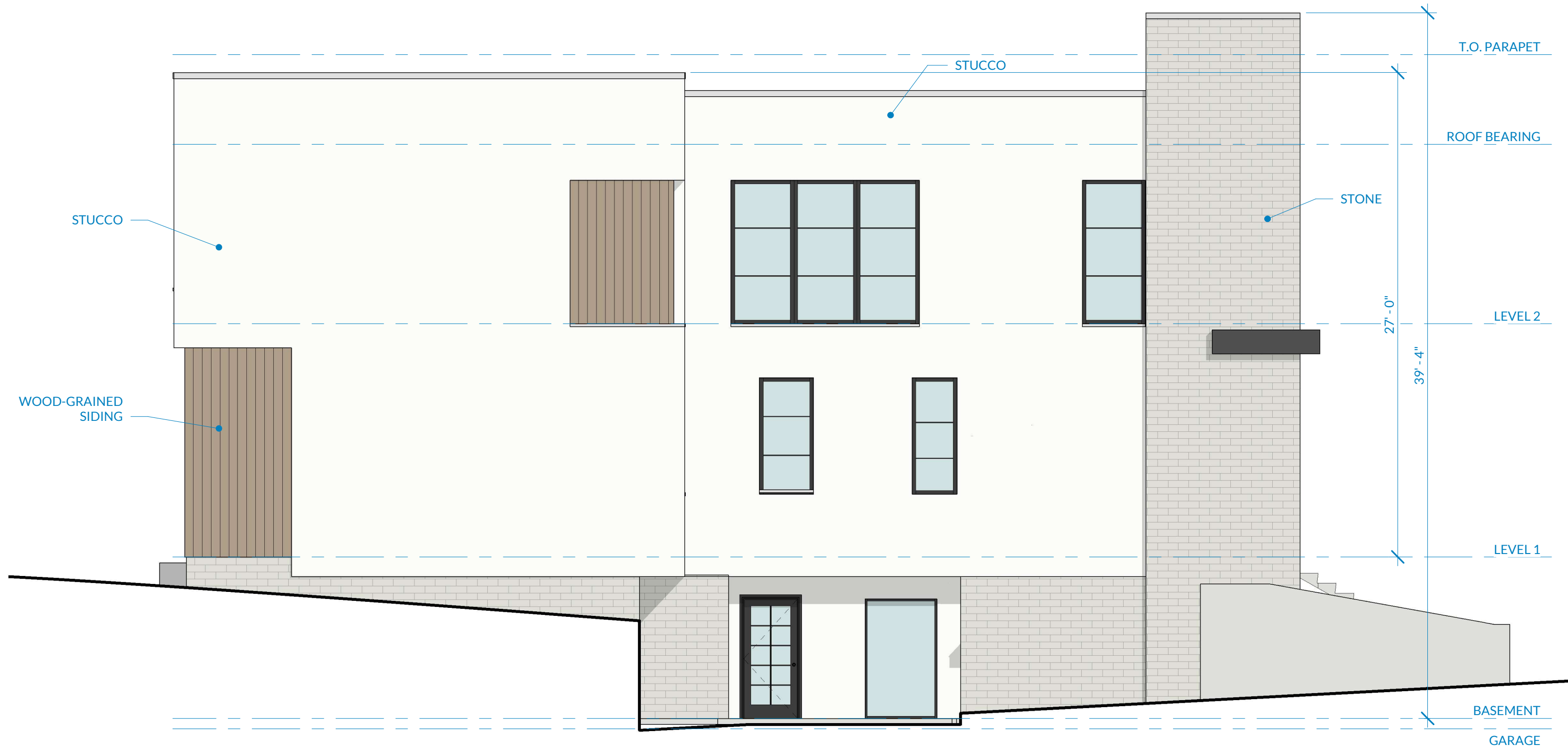
2 LOT 2 - EAST EXTERIOR ELEVATION (SIDE) 3/16" = 1'-0"
