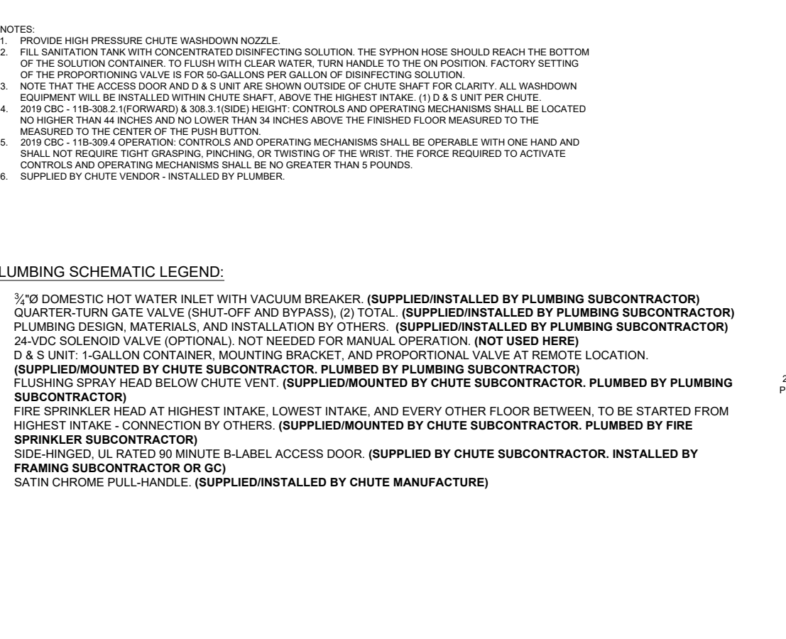
7 FIRE SPRINKLER DETAILS AND CHUTE SANITATION UNIT
