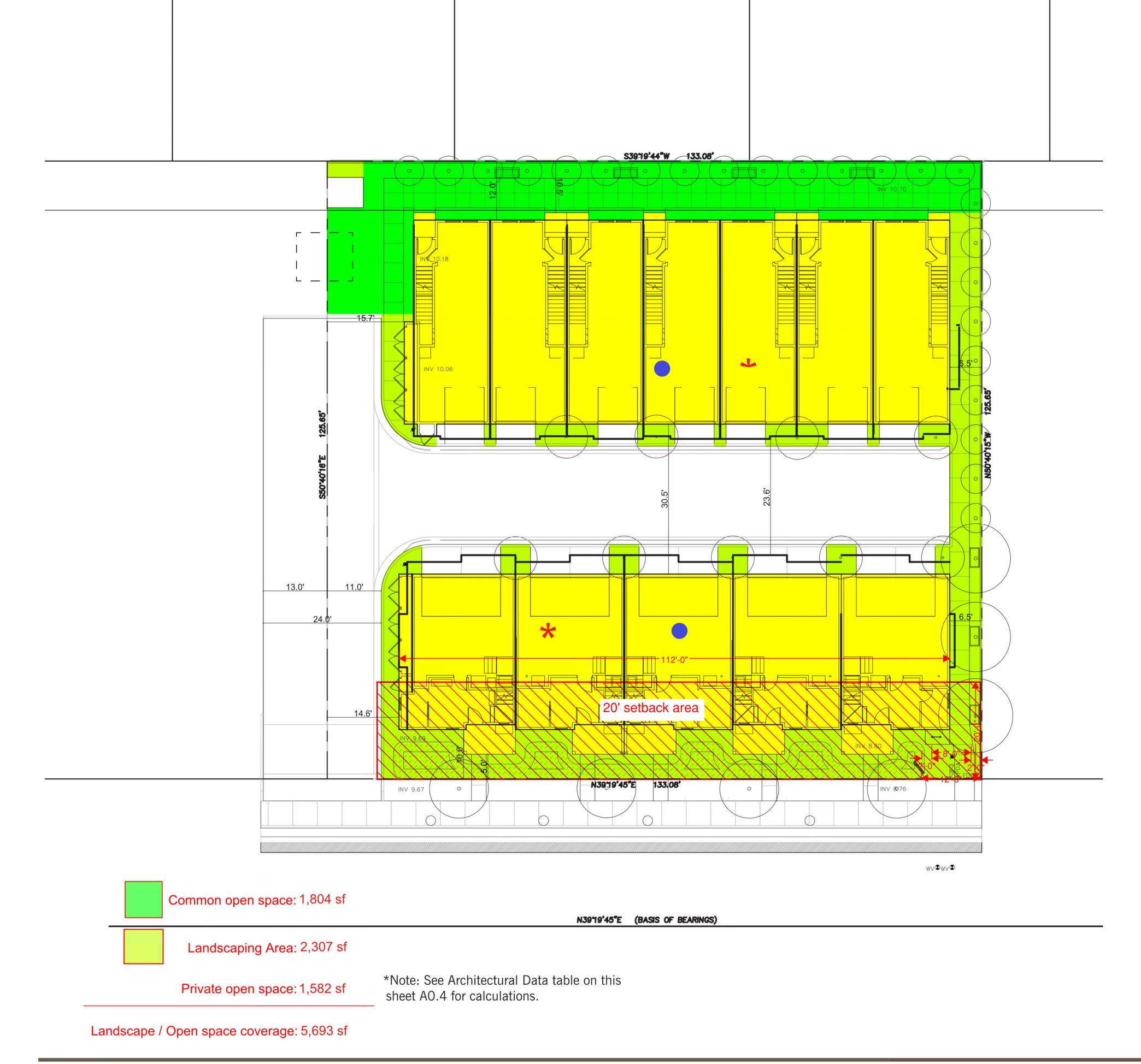
SITE PLAN WAIVER DIAGRAM 3 - MINIMUM SETBACKS, FRONT YARD - PAMC Sec. 18.13.040(a)
