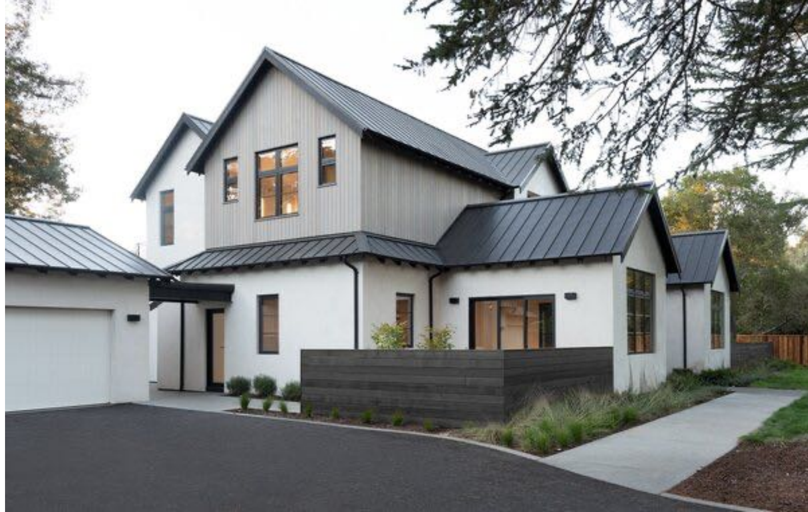
STANDING SEAM METAL ROOFING
