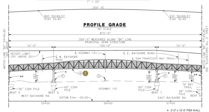
PRINCIPAL SPAN DEVELOPED ELEVATION
