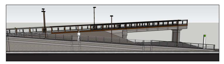
ACCESS RAMP WALL ELEVATION
