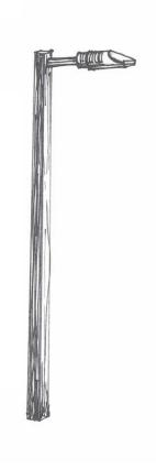
Pedestrian scale poles with adjustable led modules and field installable cutoff provides lighting at Western Approach of pathway.
