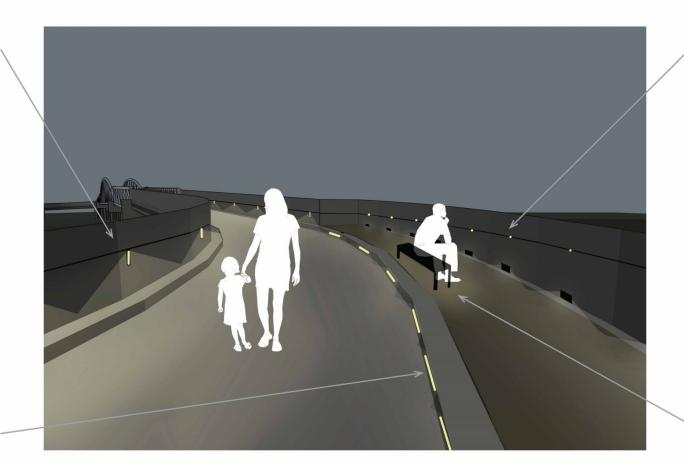
Lighting elements Integrated into railing at overlook to reduce visual interference to marshlands
