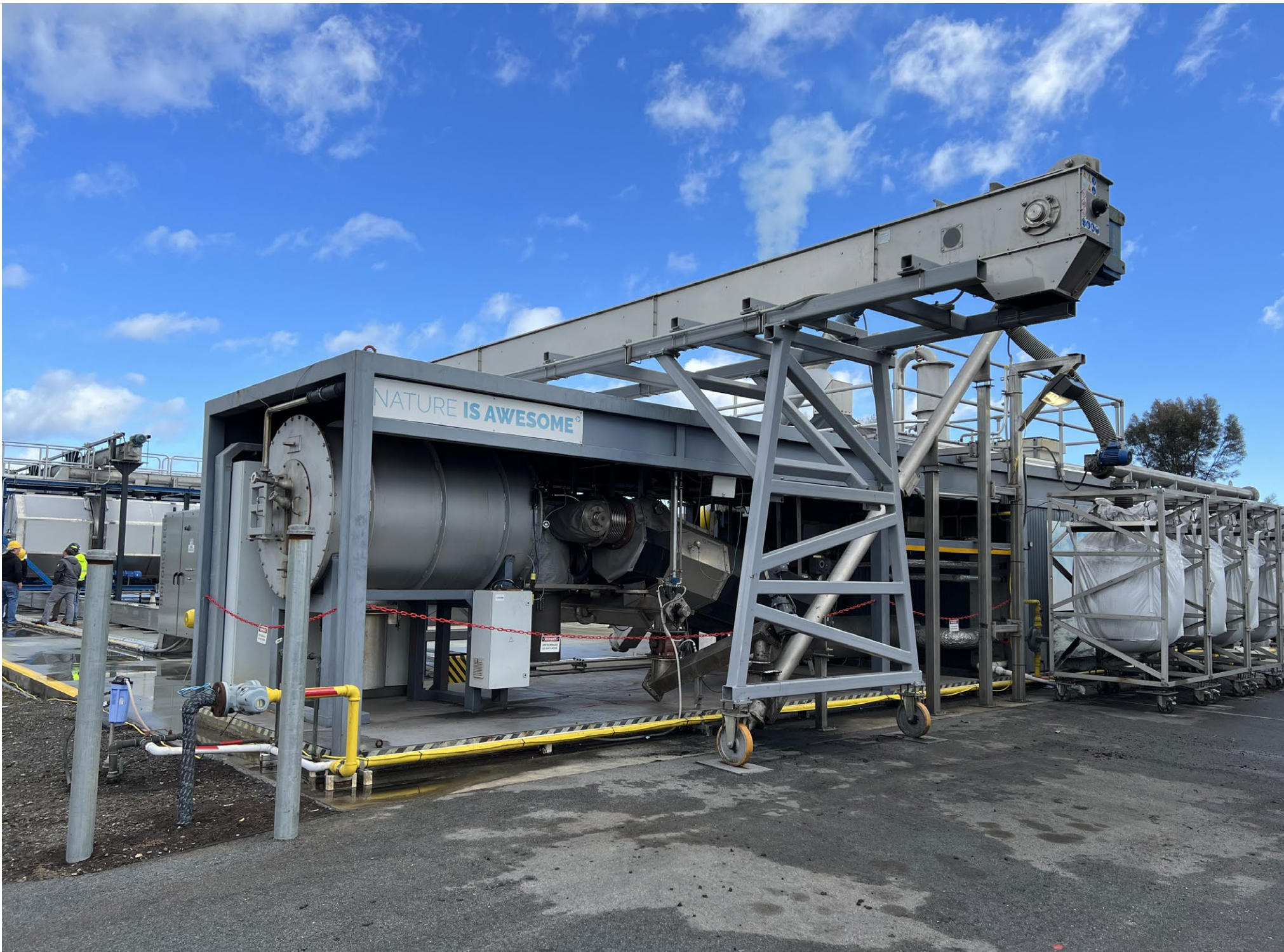
Dryers and Pyrolysis System.
