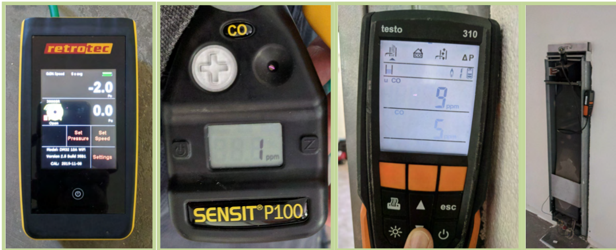
Figure 8: (from left to right) Diagnostic testing results showing -2.0 pa depressurization, 1ppm ambient CO, 5ppm CO in flue gas, and image of wall furnace testing
