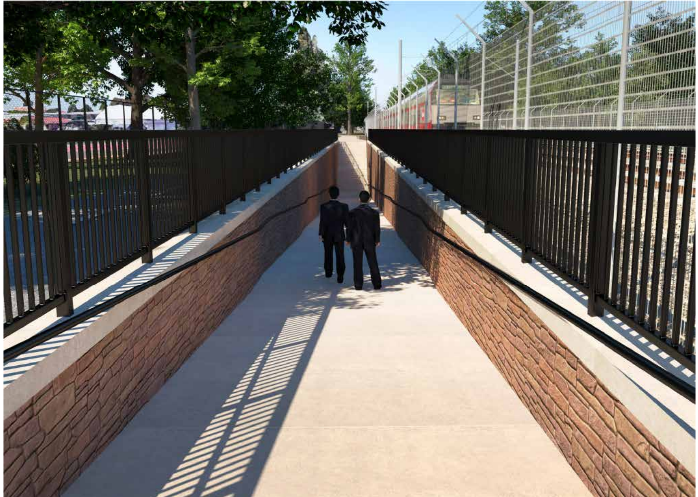
2 Example 12' Wide Ramp at 7% Grade Parallel to Caltrain Tracks
