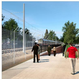
1 Example 12' Wide Ramp at 7% Grade to Tunnel
