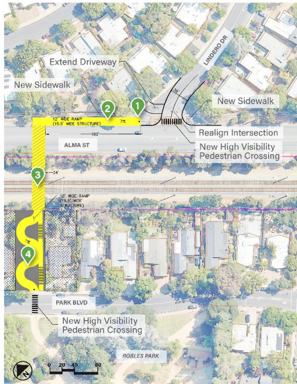
1 Example 12' Wide Ramp at 7% Grade to Tunnel
