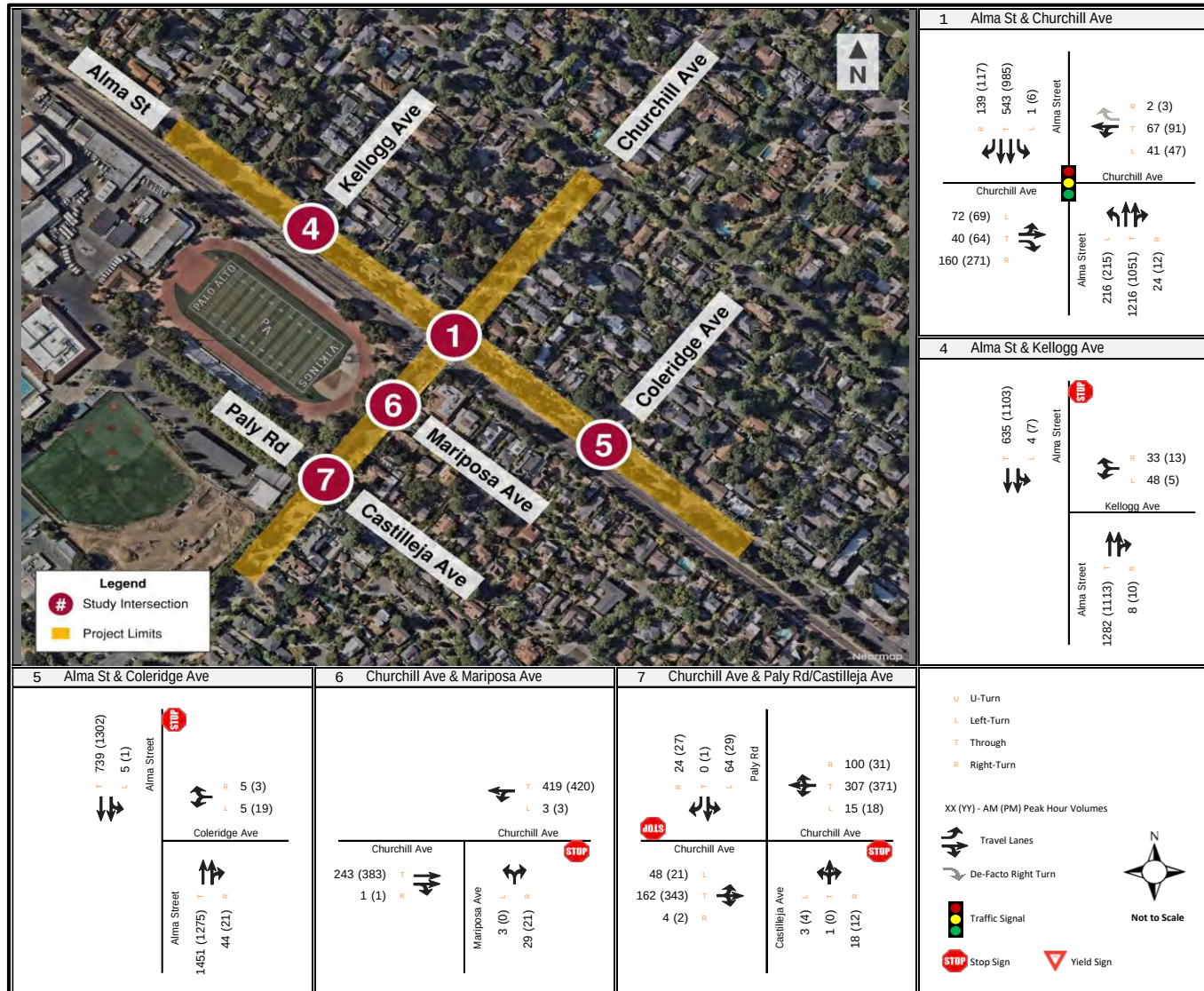
Figure 6. Existing Intersection Lane Configurations and Demand Volumes – Churchill Ave
