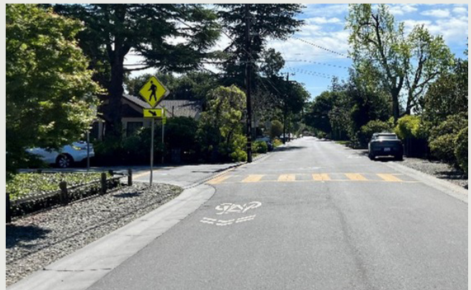
Image 10: Existing Sharrow Pavement Marking
